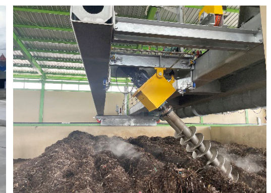
The compost plant is 100 meters long and can process up to 50 tons of food waste per day, producing 17 tons of compost.
